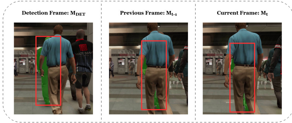
Figure 4: Three masks (in green) at different time instants for a person mostly occluded, which are the input to MIR. The real position of the person is represented by bounding boxes. The sequence belongs to the MOTSynth dataset.
