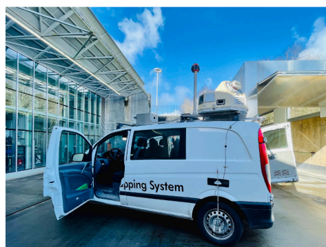
(a) The mobile mapping system used for data acquisition
