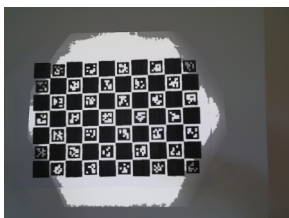
Fig. 7. The calibration board used for camera calibration and registration.
