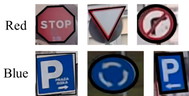
Fig. 12. Example of traffic signs segmentation with different colors and shapes. There are no brown and green traffic signs in the Santiago dataset.
