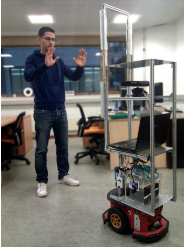
Figure 7.12: The robot is detecting a human who stopped in front of it. The human raises his hands up towards the robot. This allows the robot to detect the hands and start tracking them, in order to recognise commands from the human.
