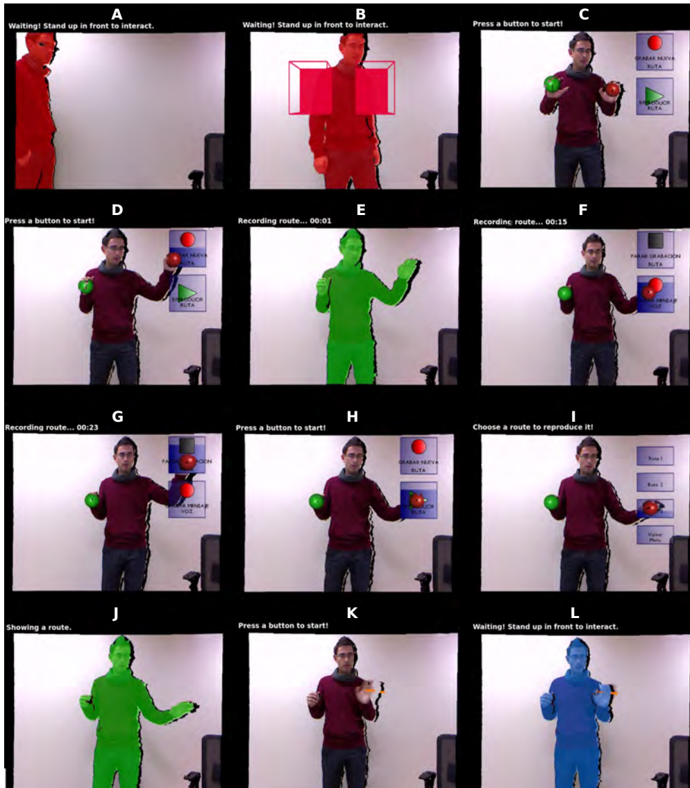
Figure 7.14: Augmented reality graphical user interface (AR-GUI) displayed on the robot's screen. We can see how a user enters the robot's field of view, initialises his hand positions and starts giving commands to the robot.
