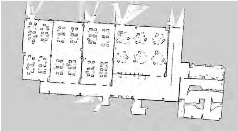
Figure 5.16: Example of a laser occupancy map M_O . White represents free space, black represents occupied space, and grey represents unknown space.
