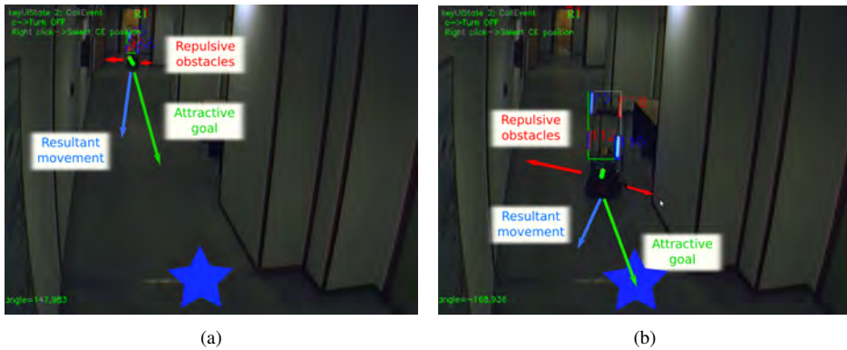
Figure 4.5: Example of support of robot navigation from a camera using a Potential Fields Controller. The star represents the position that the robot has to reach. The red arrows represent repulsive forces exerted from the obstacles in the environment. The green arrow represent the attractive force towards the goal position. The blue arrow represents the resultant force, which indicates the movement direction.
