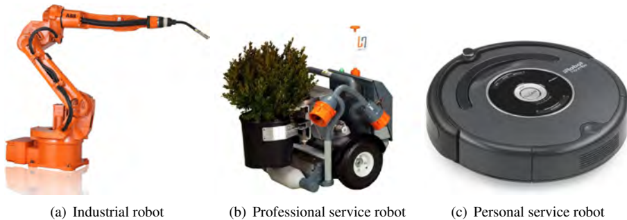
Figure 1.1: Examples of the different types of robots: industrial, a welding robot from ABB; professional, a pick and place agricultural robot from Harvest Automation; and personal robots, a vacuum cleaner Roomba from iRobot.
