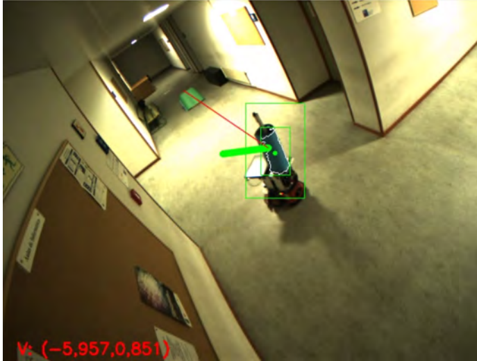
Figure 3.1: Robot detection with a blue passive marker. We represent: 1) the centroid of the robot blob with a green dot, 2) the area where the blob is detected with a small green box, 3) the area where the marker will be searched in next image frame with a big green box, 4) the direction of movement of the robot with a green line, and 5) the direction where the robot should aim (call event) with a red line.
