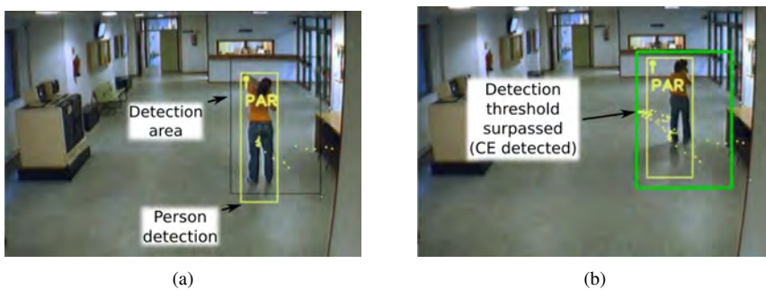
Figure 3.12: Detection of a person standing in a certain area. a) before a certain time threshold, and b) after a certain time threshold (call event triggered).
