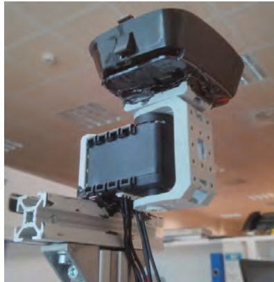
Figure 7.6: The Dynamixel AX-12A installed on top of the mast that holds the camera. This configuration allow us to pan the robot's camera.
