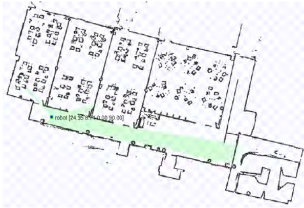
Figure 5.4: Representation of an occupancy map, a robot (blue square) and its 2D laser signature (green area).
