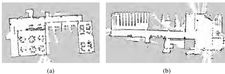
Figure 5.37: Occupancy maps created using GMapping SLAM algorithm for the third set of experiments: a) basement floor map, b) ground floor map.
