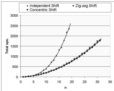
Fig. 6. Total operations (number of shift and decomposition templates) versus order of neighborhood with different shift strategies.
