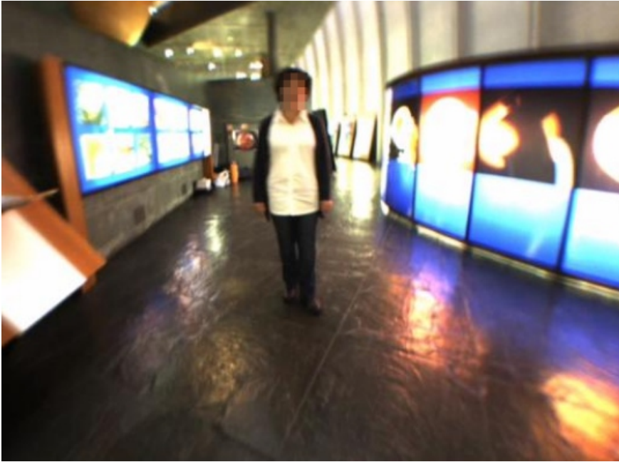
Figure 2.24: Frame captured from the demonstrations at the Domus museum (A Coruña) when the robot was following the person in the centre of the image. In this frame it is possible to observe how several light sources are causing many reflections.
