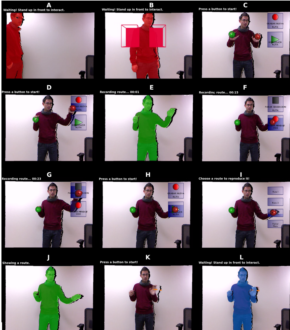
Figure 3.6: Augmented reality graphical user interface (AR-GUI) displayed on the robot's screen. We can see how a user enters the robot's field of view, initialises his hand positions and starts giving commands to the robot.
