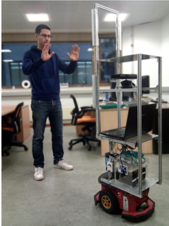
Figure 3.2: The robot is detecting a human who stopped in front of it. The human raises his hands up towards the robot. This allows the robot to detect the hands and start tracking them, in order to recognise commands from the human.
