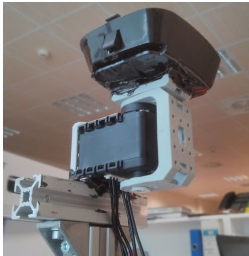
Figure 2.6: The Dynamixel AX-12A installed on top of the mast that holds the camera. This configuration allow us to pan the robot's camera.
