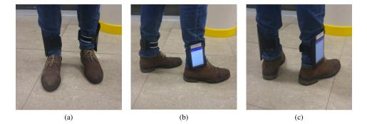
Figure 3.5: Sports armbands holding the mobiles of the legs. (a) Frontal view; (b) side view; (c) rear view.
