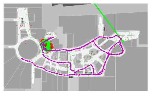
Figure 6.2: Example of a trajectory detected by the system. The purple dots and line represent the estimated positions and trajectory. The green area is a particle cloud around the user position at that moment of time.
