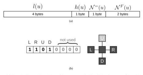
Figure 4.6: Example of data packing. (a) Data of the automaton packed into 64 bits, (b) structure of the variable  $\mathcal{N}^{=}(u)$  using 4-connectivity packed in 1 byte.
