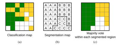
Figure 3.3: Example of majority vote between a classification map with three classes (green, yellow and white) in (a), and a segmentation map with three regions (A, B, and C) in (b). The result of the MV is illustrated in (c).
