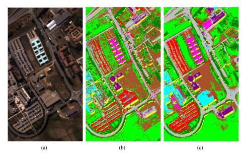
Figure 3.12: WT–EMP on the University of Pavia dataset: (a) true color representation, (b) SVM classification map, and (c) WT–EMP classification map.
