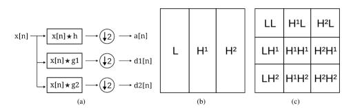
**Figure 2.16:** 2D Double-Density DWT: (a) low-pass and high-pass filters diagram, (b) separable transform applied to the rows of an image, (c) separable transform applied to the columns of (b). (\* stands for circular convolution).
