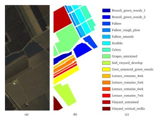
Figure 2.26: Salinas Valley dataset. True color representation (a), reference map with sixteen classes of interest (b), and name of the classes (c).
