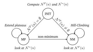
Figure 4.4: Three-state cellular automaton implementing Hill-Climbing algorithm [64].
