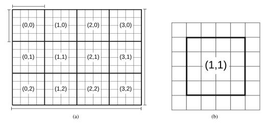
Figure 4.1: Example of grid/tiling model in CUDA: (a) grid of  $16 \times 16$  threads divided into blocks (tiles) of  $4 \times 4$  threads, and (b) a block extended with a border (apron) of size one.
