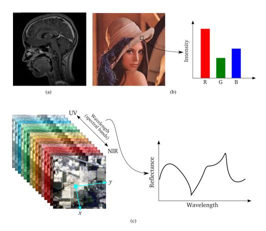
Figure 2.1: *n*-dimensional images. (a) 2D slice of a CT scan, (b) color image and the intensity of the RGB channels, and (c) hyperspectral image and the different wavelengths responses of a pixel vector.
