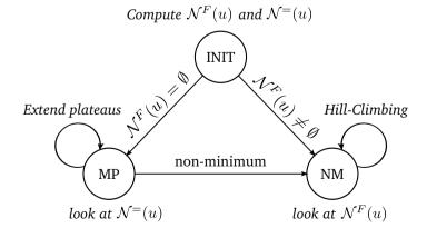
Figure 3.6: 3-state cellular automaton implementing Hill-Climbing algorithm [64].
