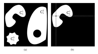
**Figure 2.11:** Example of a connected opening. (a) Binary image with three connected components named  $C_1^1, C_1^2$ , and  $C_1^3$ , and (b) the connected opening  $\Gamma_x$  indicated by the intersection of the dot lines.
