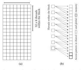
Figure 5.10: 1D-DWT by columns kernel: data read from global to shared memory by a block of  $32 \times 8$  threads (a), and shared memory access pattern for each thread within the block (b). Each square in (a) represents  $4 \times 1$  data items in the shared memory.
