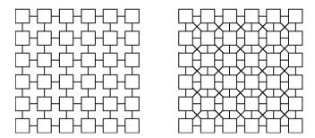
Figure 2.7: Cells arranged in a regular grid of two dimensions. Cells are connected to four (left) and eight (right) adjacent neighbors.
