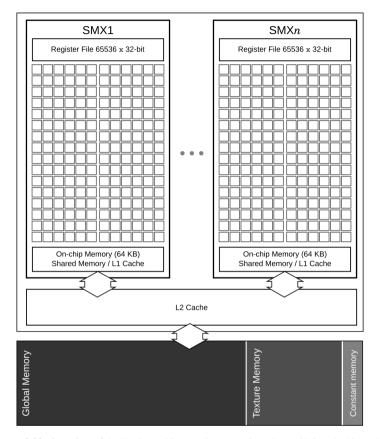
Figure 2.20: Overview of the Kepler architecture incorporating a L1 and L2 cache hierarchy.
