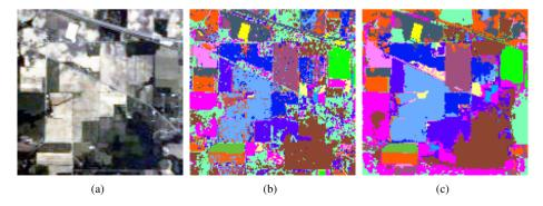
Figure 3.14: WT–EMP on the Indian Pines dataset: (a) true color representation, (b) spectral classification map with SVM, (c) WT-EMP classification map.
