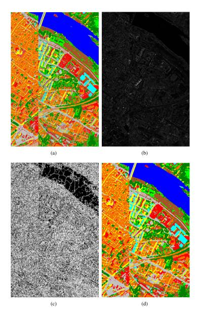
Figure 3.9: CA–WSHED–MV on the Pavia City dataset: (a) SVM classification map, (b) RCMG, (c) CA–Watershed segmentation, (d) final classification by majority vote.
