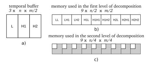
Figure 5.8: 2D-DWT global memory requirements (indicated with a white background), for an image of  $n \times m$  pixels, using a set of three filters and two levels of wavelet transform. (a) Temporal buffer for separable wavelet transform, (b) and (c) memory used in the first and the second level of decomposition, respectively.
