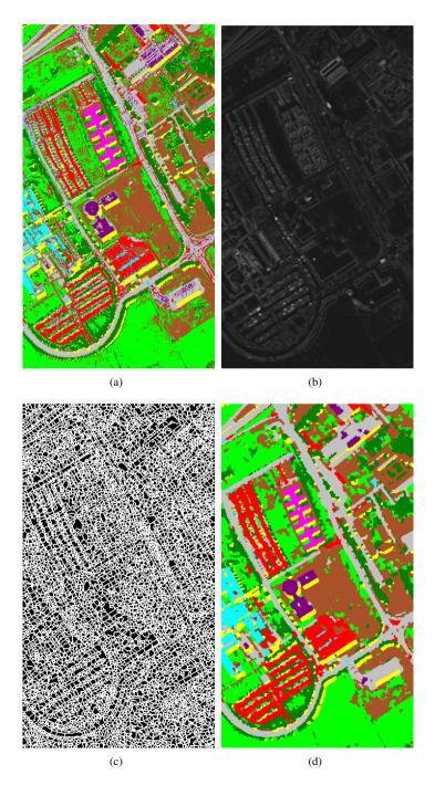
Figure 3.8: CA–WSHED–MV on the University of Pavia dataset: (a) SVM classification map, (b) RCMG, (c) CA–Watershed segmentation, (d) final classification by majority vote.
