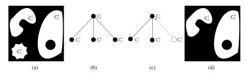
Figure 2.12: Example of a attribute opening. (a) Binary image with three connected components named  $C_1^1$ ,  $C_1^2$ , and  $C_1^3$ , (b) tree representation of the image, (c) attribute filtering removing a node of the tree, and (d) the final result.
