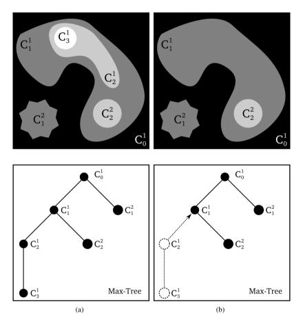
**Figure 4.14:** Example of a greyscale attribute opening. (a) Greyscale image with five connected components (the grey level is indicated by the subscript, and the *i*-th component within a level is indicated by the superscript) and the corresponding max-tree, (b) result of the attribute opening on the greyscale image and the pruning of the max-tree.
