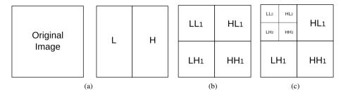
Figure 2.15: Separable 2D-DWT applied to the rows of the image (a) and then, to the columns (b), and the result of 2 levels of decomposition (c).
