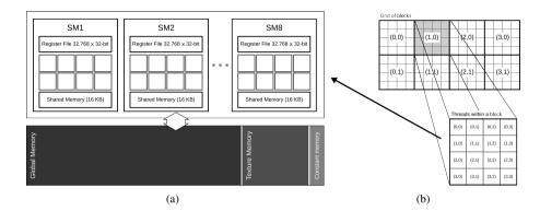
Figure 2.19: CUDA. (a) Overview of G80 architecture, (b) grid of blocks and block of threads scheduled to any of the available SMs.
