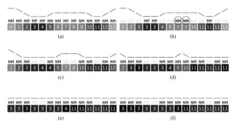
Figure 3.7: CA–Watershed based on Hill-Climbing algorithm. Example of 1D image represented as a terrain with dashed lines and as grey values with the squares: a) pixels are sequentially labelled and states are initialized, b) MP updating stage where two pixels change their state to NM c) to f) the automaton evolves only with the NM rules.
