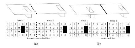
Figure 4.11: An image of  $4 \times 16$  pixels displayed as a topographical relief (top) and the map of distances when the watershed is computed using asynchronous blocks (a), and the map of corrected distances (b).
