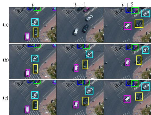
Figure 1: Comparison of (a) a multi-object tracking system lacking motion estimation between detections, (b) SiamMT [4], and (c) our proposal (SiamMOTION). Notice how (a) is unable to handle all frames and (b) does not detect changes in the aspect ratio of the objects.
