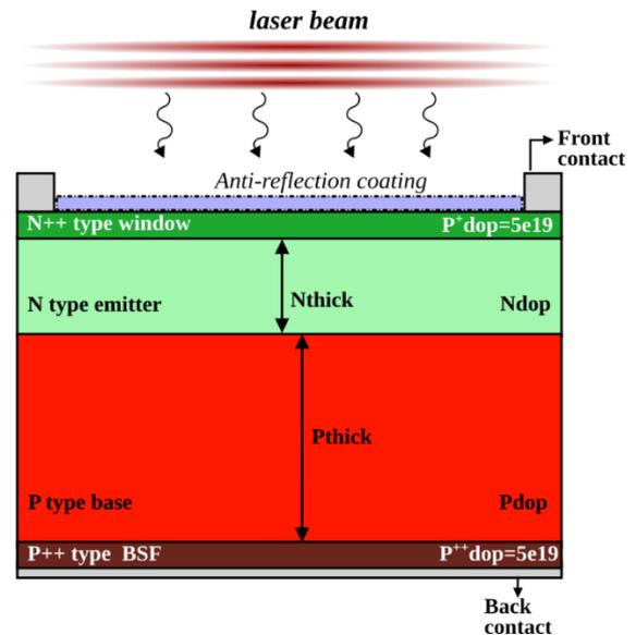
Fig. 1. 2D scheme of the hLPC architecture. The thickness and doping values of the window layer and back surface field (BSF) layer are fixed in the optimization process.
