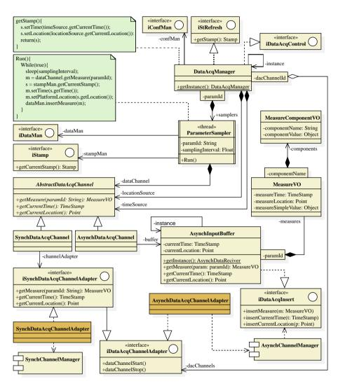
Figure 3.3: UML Class Diagram of component DataAcquisition.
