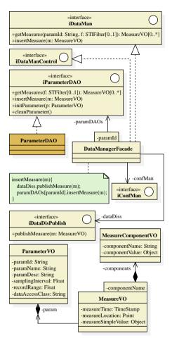
Figure 3.5: UML Class Diagram of component DataManager.
