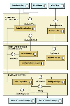
Figure 3.1: GeoDADIS component architecture.
