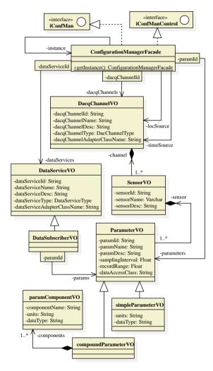
Figure 3.4: UML Class Diagram of component ConfigurationManager.
