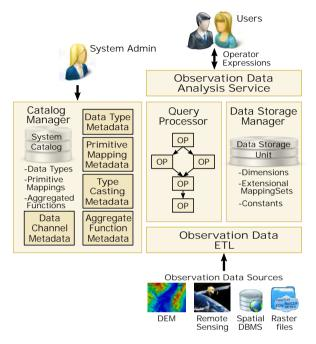
Figure 5.1: SODA Prototype Architecture.
