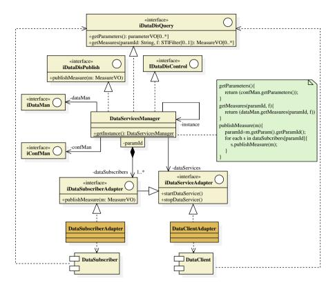
Figure 3.2: UML Class Diagram of component DataDissemination.
