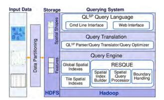
**Figure 2.1:** Architecture of Hadoop GIS. source: *Aji et ál., in Proc. VLDB Endow.*, 2013 [5].
