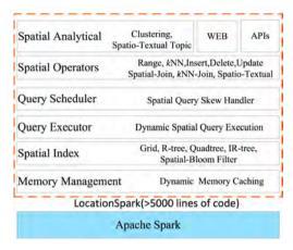
Figure 2.5: Architecture of LocationSpark. source: *Tang et ál., in Proc. VLDB Endow., 2016* [95].
